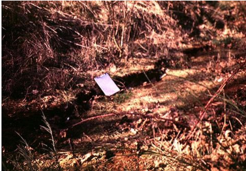
Figure 7: Fresh tension crack located above head scarp of the Hilltop Avenue landslide, located at the dead end of Hilltop Avenue in the southwest section of the study area ( 8\frac{1}{2} \times 11 inch field notebook for scale).
