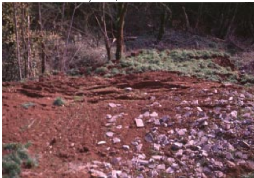
Figure 7: Fresh tension crack located above head scarp of the Hilltop Avenue landslide, located at the dead end of Hilltop Avenue in the southwest section of the study area ( 8\frac{1}{2} \times 11 inch field notebook for scale).
