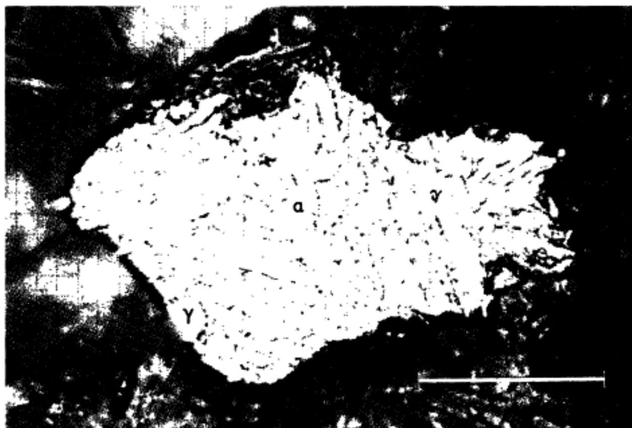
Fig. 7 Zoneless plessite ( \alpha + \gamma ) grain in Kernouvé. Scale bar = 25 \mu\text{m} ; 2% nital etch. Note the pseudo-Widmanstätten pattern.
