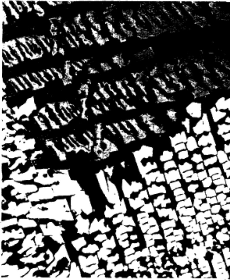
Fig. 7 A crossed-polar view of an ultra-thin section of a type S deep-sea spherule. The width of the image is 100 \mu\text{m} .
